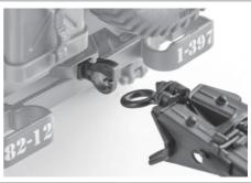
Rotate the turret brackets on both sides of the wheel down 180°;
